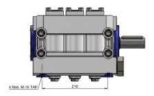
Note: All dimensions are in mm & weight of bare pump is around 85 Kg approx.
