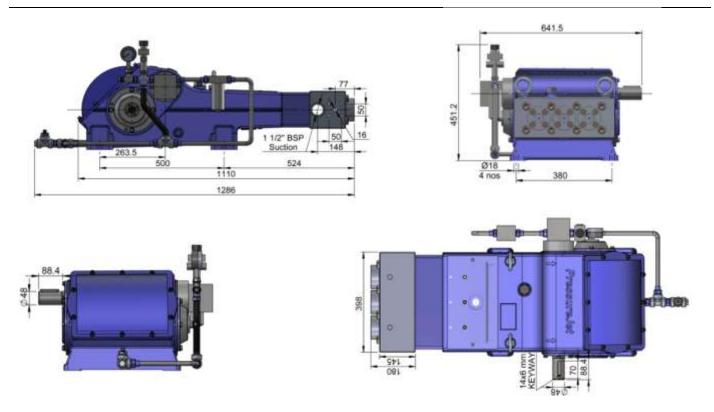
Note: All dimensions are in mm & weight of bare pump is 410 Kg approx.
